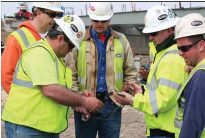
Crew members inspect a lanyard for evidence of damage after testing the fall arrest system on March 19th at a bridge on Beltline Road in Rockford. Pictured here are Gene Woodley, Curt Ihrig, John McClelland, Shawn Meier and Brian Balles.
